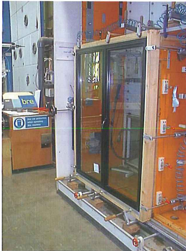
Figure A1. Smart Systems side hung casement 'Evolution' window in the BRE Test rig 'G'
